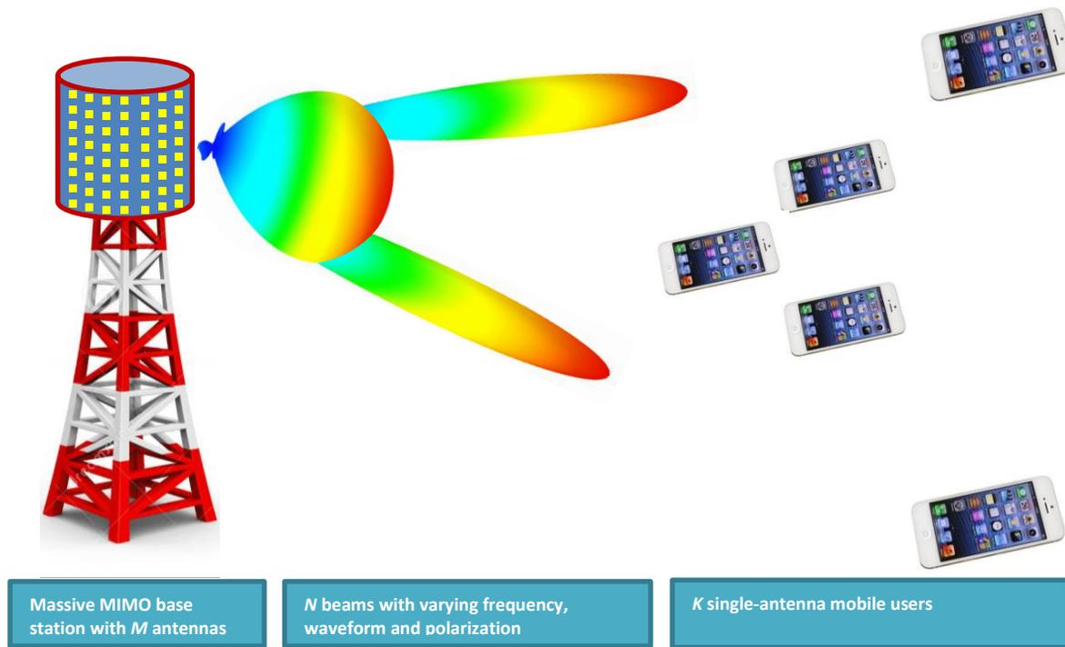
Figure 1: Conceptual drawing of a multi-antenna massive MIMO mm-wave 5G base station with  $M \gg K$ . Multiple beams with different shapes, waveforms, frequency and polarization can be created simultaneously. The antenna system includes radiating elements, RF electronics and signal-processing.
